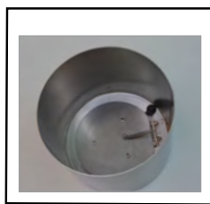
Pressure relief flap with an additional relieving spring as a safety measure in the event of faults
